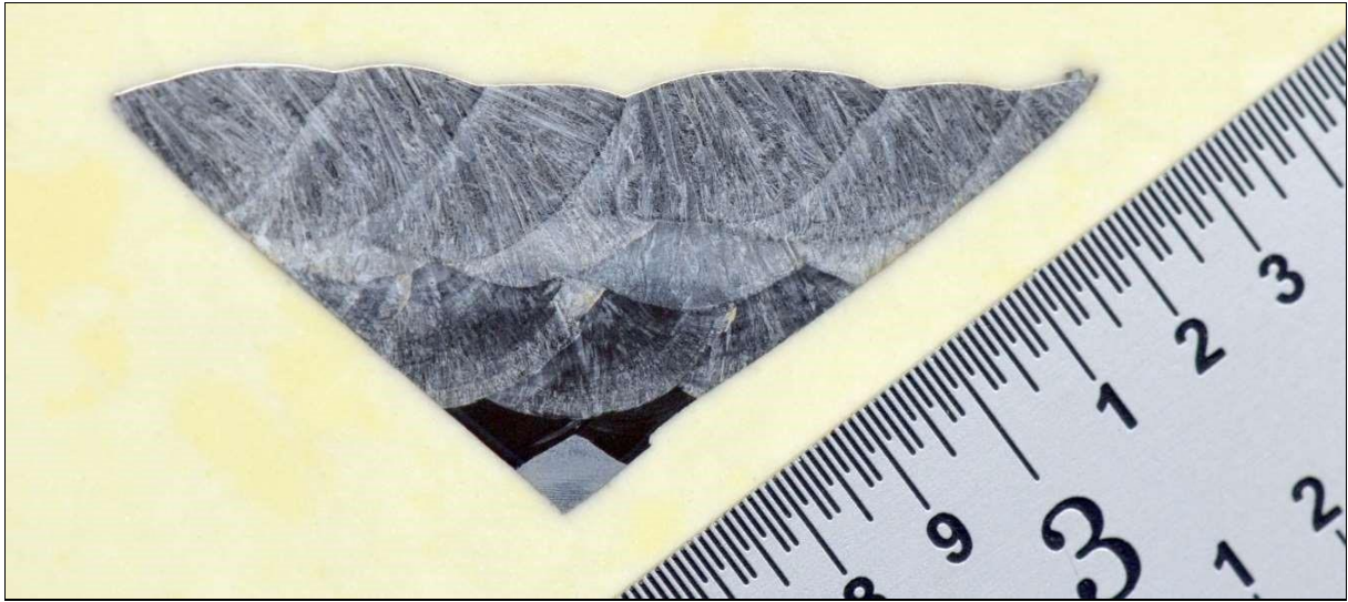
FIGURE 3. Etched cross section through Control sample. (NAOH Electrolytic etchant, Scale 0.01" divisions)
