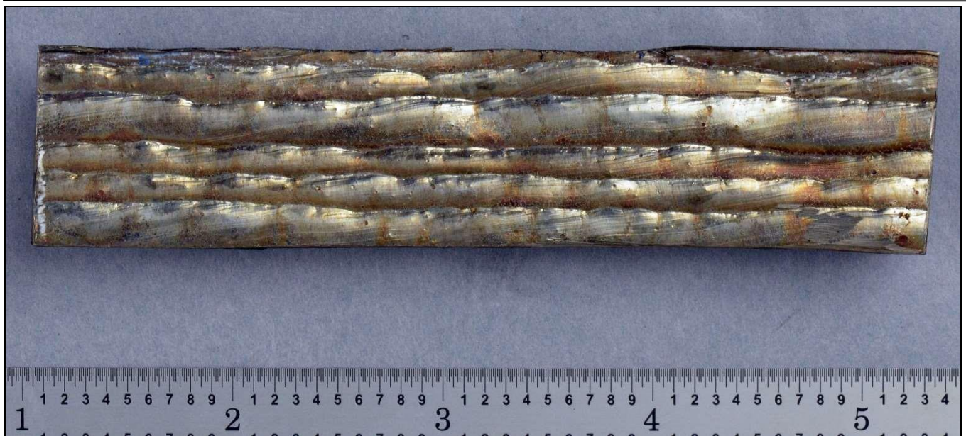
Figure 1. Photograph showing the surface of the “Control” overlay sample as-received (Scale 0.01” divisions).
